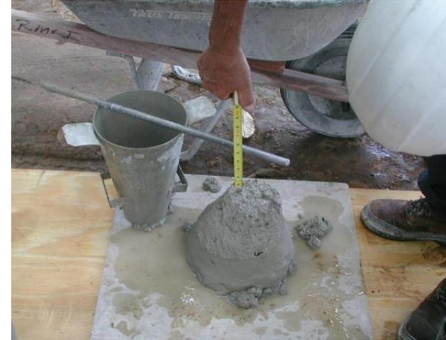
ASTM C143 Slump (Asentamiento)
